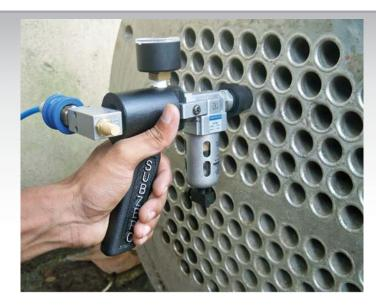
The vacuum leak tester SVLD-3000 is a very quick, easy & precise method of testing damage or leaky tubes of boilers, condensers, & heat exchangers. Also it is very economical & fast method compare to hydro test for locating
